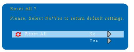
2. Press reset button on the remote control or the button on the control panel to reset the OSD Menu values. Press the ESC button or ignore the message to exit the Reset All function without changing any settings.
