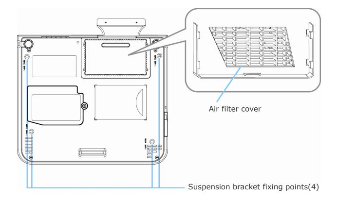
**1.** Suspension bracket fixing points (4 points)
