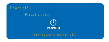
2. Press the power button again and the projector will enter cool-down mode. The lamp shuts off, the lamp indicator flashes red, and the fans continue to run for approximately two minutes. During the cool down sequence the projector will not respond to any control panel or remote control buttons.
